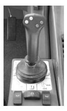
To extend the boom, move the joystick right; to retract the boom, move the joystick left. To raise the boom, move the joystick rearward; to lower the boom, move the joystick forward.
