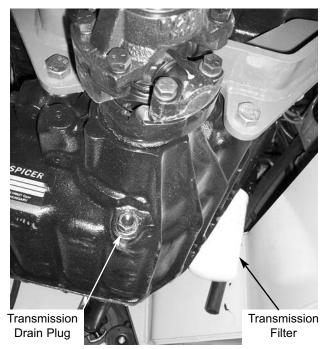
Operate the machine long enough to warm up the transmission oil. Shut off the engine. Access to filter and drain plug is from underneath the machine. Proceed as follows:
