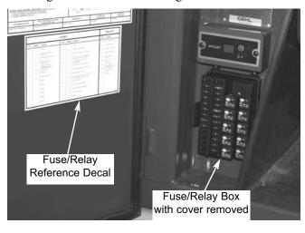
**Fuse and Relay Functions:** The cover of the fuse box has a diagram indicating the position of the fuses and relays inside the box. Remove the cover to gain access to the fuses and relays. Refer to the illustration and following descriptions for the fuse and relay functions.
