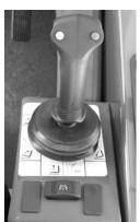
boom, move the joystick left. To raise the boom, move the joystick rearward; to lower the boom, move the joystick forward.
