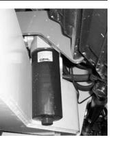
Insert the new element onto the housing and replace the cover.
