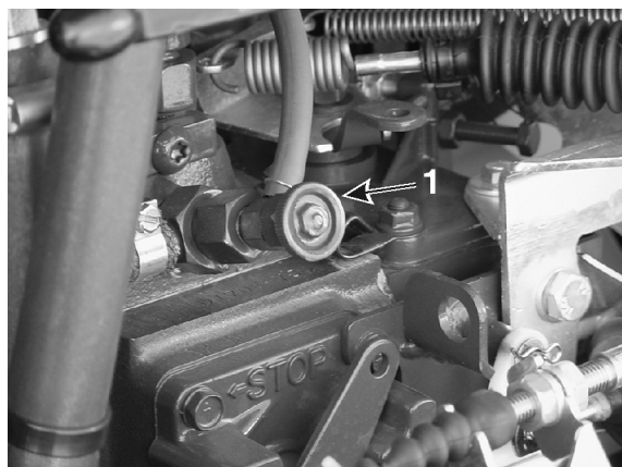
Figure 4-8 Bleeding Air from Fuel System on Machine with Serial Numbers Before AD00001
