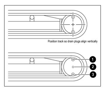
Figure 4-20 – Plugs for Drive Oil Check/ Change
