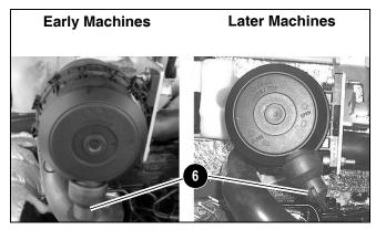
Figure 4-5 – Air Filter Dust Valve
