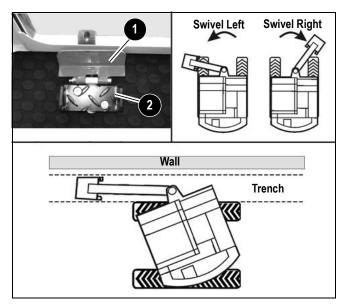
Figure 3-17 - Boom Swivel Controls
