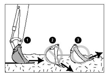
Figure 3-31 – Proper Bucket Position
