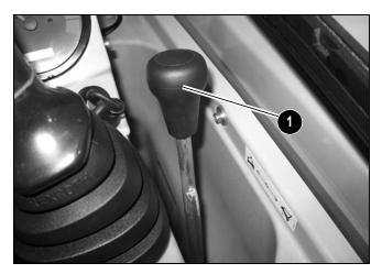
Figure 3-36 – Dozer Blade Lever
