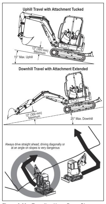
Figure 3-29 – Traveling Up or Down Slopes
