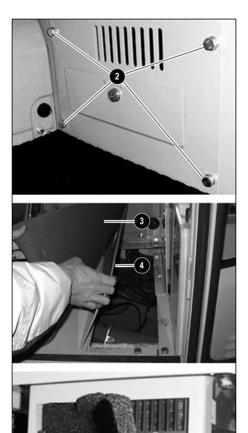
Figure 4-23 – Accessing the Heater Filter
