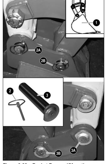
Figure 3-39 - Bucket Removal/Mounting
