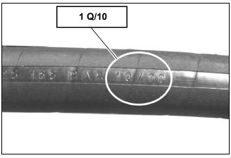
Figure 4-15 Hydraulic Hose Manufacture Date
