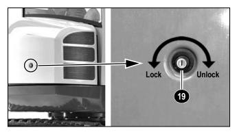
Figure 3-6 - Engine Hood Lock
