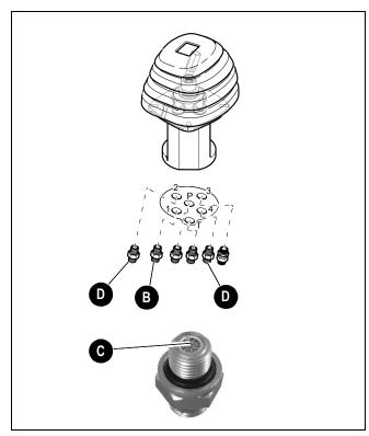
Figure 4-14 Pilot Control Filter/Restrictor
