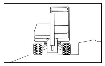
Figure 3-28 – Working from a Level Area
