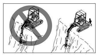
Figure 3-35 – Machine Position for Deep Excavating
