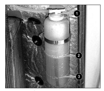
Figure 4-11 – Coolant Expansion Reservoir
