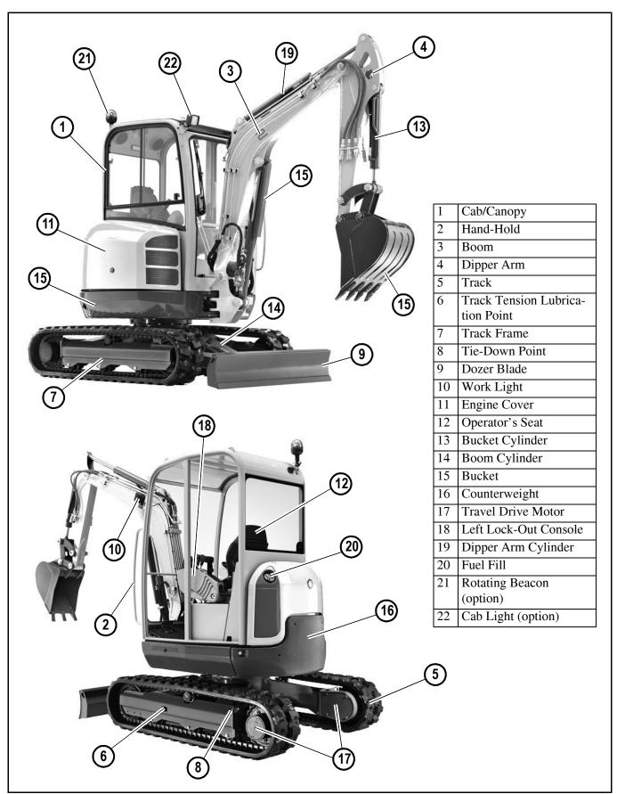
Figure 1-3 - Component Identification
