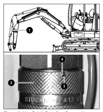
Figure 3-41 – Quick Coupling Connections
