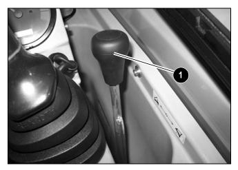
Figure 3-8 – Dozer Blade Lever
