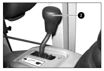
Figure 3-9 – Throttle Lever
