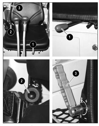
Figure 3-18 - Seat Adjustment
