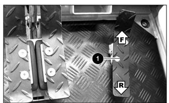
Figure 3-42 - Auxiliary Hydraulics Control
