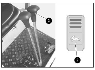
Figure 3-11 – High-Speed Switches
