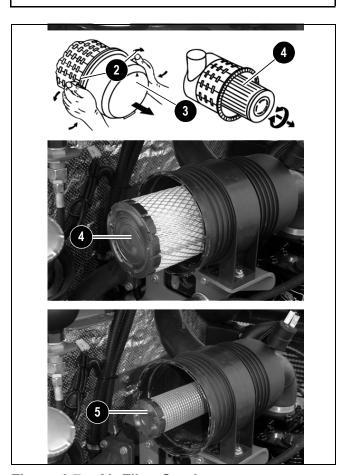
Figure 4-7 – Air Filter Service
