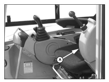
Figure 3-1 – Operator's Left Console in Lockout Position
