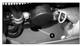
Figure 4-3 – Engine Oil Drain Access
