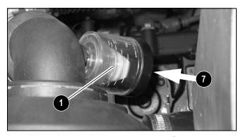
Figure 4-6 – Air Filter Restriction Gauge
