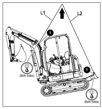
Figure 3-44 - Machine Lifting Points
