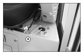
Figure 3-2 - Left Console Height Adjustment
