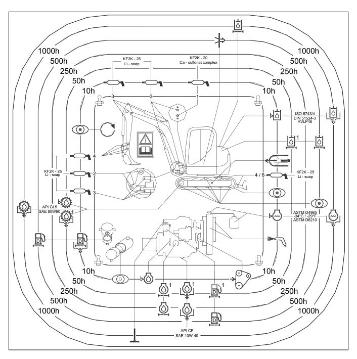
Note: Maintenance label is located on cab rear window or inside right canopy wall.
