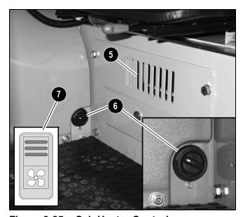
Figure 3-25 – Cab Heater Control
