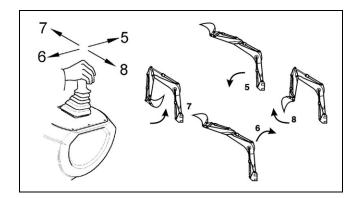
Figure 3-14 – SAE Right Joystick
