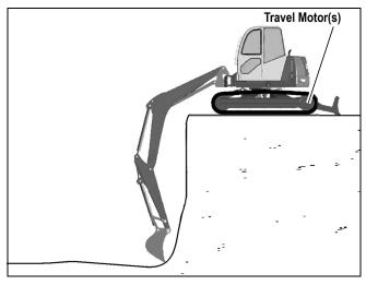
Figure 3-27 – Machine Position for Edge Excavating
