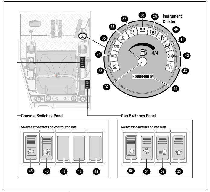
Figure 3-4 – Instrument Panel, Switches and Indicators
