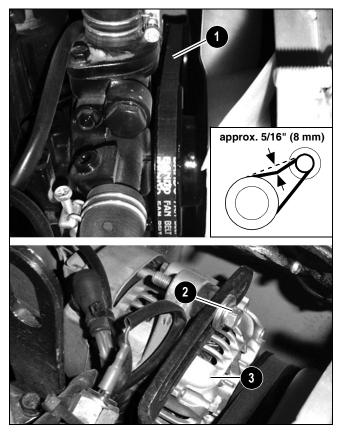
Figure 4-17 - V-belt Tension
