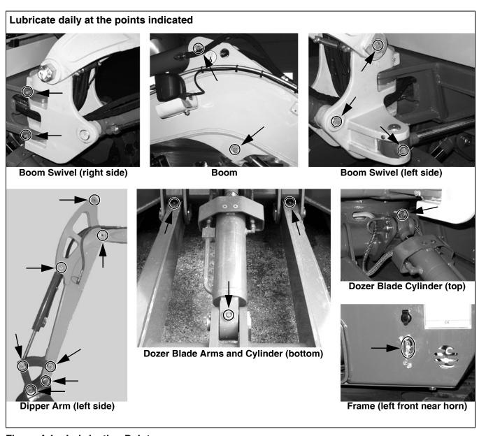
Figure 4-1 – Lubrication Points
