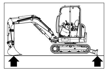
Figure 4-21 – Track Adjustment Position
