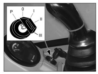
Figure 3-7 – Ignition Key Switch
