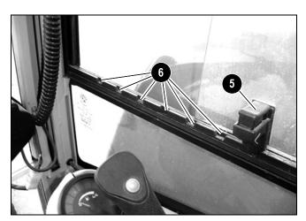
Figure 3-23 – Side Window Lock Release
