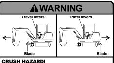
Machine travels in direction of blade when travel levers are pushed away from operator.
