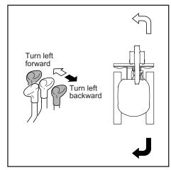
■ Steering the machine while traveling (the left and right travel levers are both tilted in the same direction)
