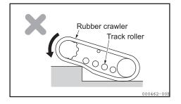
2) If the machine is traveling in reverse, clearance may also be created between the track rollers and the rubber crawlers, and between the idlers and the rubber crawlers, causing the rubber crawlers to come off.
