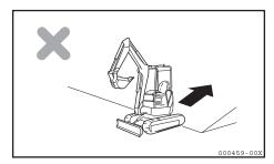
Do not travel with the crawler on one side on a slope or on convex ground (causing a machine angle of more than 10 degrees), and with the crawler on the other side on flat ground, to prevent the rubber crawler from being damaged. Be sure to travel with the crawlers on both sides on the same level surface.
