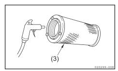
6) After cleaning, illuminate the element from inside with a light bulb and check it. If there are any small holes or thin areas, replace the element with a new one.
