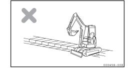
Do not steer the machine across a boundary between the flat ground and a slope, while moving backwards.
