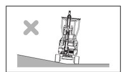
The three cases illustrated above are those which could cause the rubber crawlers to loosen. In addition, do not subject the machine to such ground conditions as are illustrated in the figure at the right.
