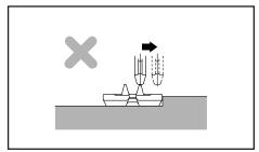
Changing the travel direction of the machine under the condition illustrated will cause the rubber crawlers to come off.
