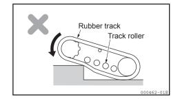
2) If the machine further travels in reverse, clearance may also be created between the track rollers and the idler and, the rubber track, causing the rubber track to easily come off.
