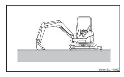
2) Lower the attachment onto the ground.
