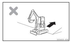
Do not travel with the track at one end on a slope or on convex ground (at a machine inclination angle of approximately more than 10 degrees), with the track at the other end on flat ground, to prevent the rubber track from being damaged. Be sure to travel with the track at both ends on the same level surface.
