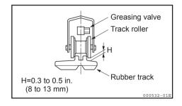
If the tension is improper, adjust it as follows:
