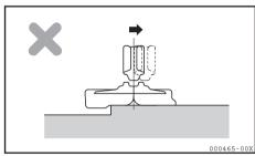
Traveling in reverse under this condition will cause the rubber track to come off.
