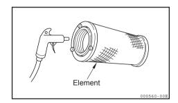
6) After cleaning, illuminate the element from inside with a light bulb to check it. If there are any small holes or thinner parts, replace the element with a new one.
