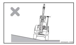
The three cases illustrated above are those which could cause the rubber track to loosen. In addition, do not steer the machine under such ground conditions as illustrated in the right figure.
