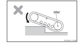
When the machine is steered while the rubber track is blocked in the transverse direction by an obstacle or the like.
