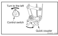
8) Remove the quick coupler from the attachment.
