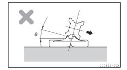
Steering the machine under this condition will cause the rubber track to come off.
