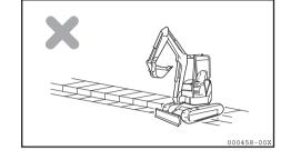
Do not steer the machine to a boundary between the flat ground and a slope while moving backward.
