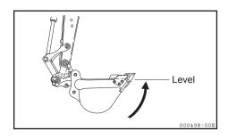
6) Turn the control switch to the mounting position on the right side, and the attachment is mounted.
