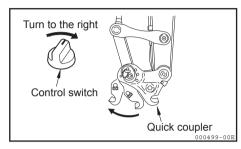
7) Only one of the bores allows the whole lock pin. Install the lock pin to that bore.
