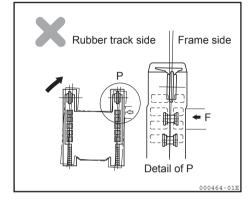
• When the idler and the track rollers are misaligned from the core metal due to rubber track misalignment.
