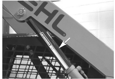
Figure 4 Lift Arm Support Device Engaged
