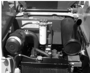
Figure 30 Hydraulic Oil Service
