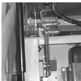
Figure 24 ROPS Lock Mechanism
