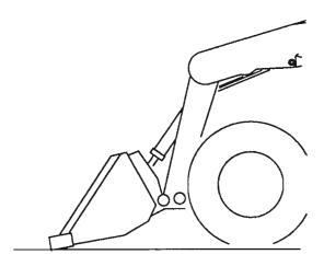
Fig. 24: Positioning Bucket for Scraping
