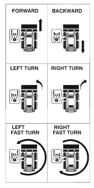
Fig. 4: Hand & Foot Loader Movement
