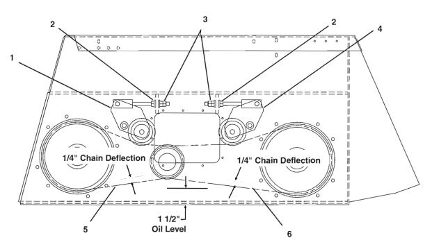
Fig. 31: Adjusting Drive Chain Tension (Left side shown, Right side Typical)
