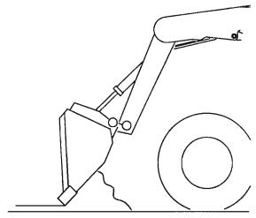
Fig. 26: Leveling with a Bucket
