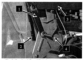
Fig. 8: Overhead Guard Unbolted, Rolled-back & Locked
