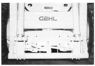
Fig. 11: Quick-Tach Lever in "Release" Position all the way to the Right (Attachment Removed for Clarity)
