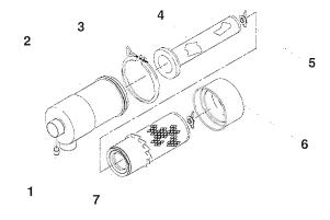
Fig. 38: Dual Element Air Cleaner
