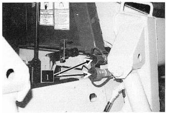
Fig. 14: Standard Flow Auxiliary Hydraulics
