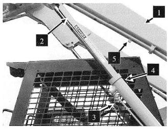
Fig. 12: Lift Arm raised & Lock "Engaged"
