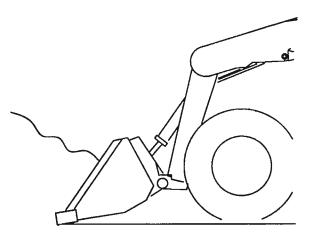
Fig. 22: Digging in Loose Materials
