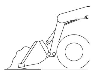
Fig. 25: Scraping with a Bucket
