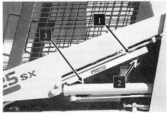
Fig. 13: Lift Arm Lowered & Lock "Stored"
