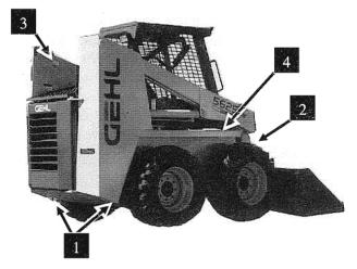
Fig. 27: Lifting & Tie Down Locations
