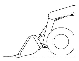
Fig. 21: Digging in Hard-packed Materials
