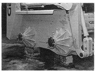
Fig. 28: Skid Loader properly Blocked (the Tires and Wheels are removed to show Blocks ).
