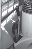
Fig. 24: High-Flow Control (Joystick controlled units)
