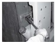
Fig. 50: Remove cooler lock bolt
