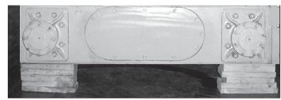
Fig. 37: Loader Properly Blocked (Tires and wheels removed to show blocks)
