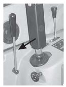
Fig. 7: Hand Throttle Lever (T-Bar, Dual-Hand & Hand/Foot controlled units)
