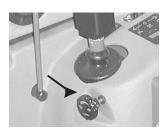
Fig. 19: Standard-Flow Control Knob (T-Bar, Dual-Hand & Hand/Foot controlled units)
