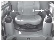
Fig. 15: Joystick Controls
