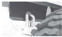
Fig. 34: Four-Point Lift Front Lift Eye
