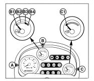
A - HOURMETER AND TACHOMETER
