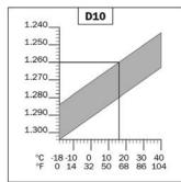
Readings above this zone indicate that the battery needs to be recharged.
