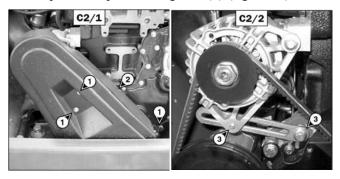
**IMPORTANT:** If the alternator belt is replaced, check the tension again after 20 hours of operation.
