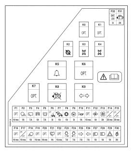
**IMPORTANT:** Replace a failed fuse with a new fuse of the same quality and capacity. Never use a repaired fuse.
