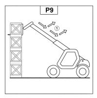
➡ If this is not possible, reverse the telescopic handler (1) very slowly and carefully to release the forks (fig. P10). Then return the forks to transport position.
