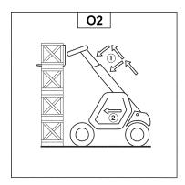
Slightly lift the load (1) and tilt the carriage (2) rearward to stabilize the load (fig. O3).
