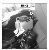
Visually check that there is no leakage at the reservoir and connections.
