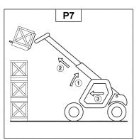
Place the load in a horizontal position and set it down on the stack by lowering and retracting the boom (1) (2) to position the load correctly (fig. P8).
