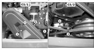
**IMPORTANT:** If the compressor belt is changed, check the tension again after the first 20 hours of operation.
