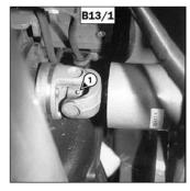
2- Grease fittings for the universal joint between the transmission and front axle (3) (fig. B13/2).
