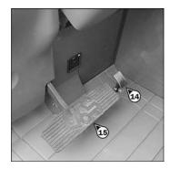
15 - SERVICE BRAKE PEDAL AND TRANSMISSION CUT-OFF
