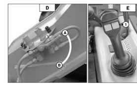
Connect the quick-connectors as needed for the attachment's hydraulic movements.
