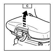
Press the left-hand button while pushing on the seat or relaxing pressure on the seat to find a comfortable position.
