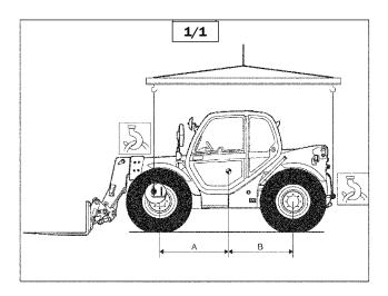
**⊃** Place the hooks in the fastening points provided (fig. 1/2 and 1/3).
