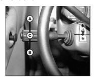
When the forward/reverse lever is in the neutral position, a mechanical lock prevents an inadvertent shifting movement.
