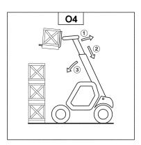
☐ If this is not possible, back up the telescopic handler (1), maneuvering very gently and carefully to release the load. Retract (2) and lower the boom (3) to bring the load into the transport position (fig. O5).
