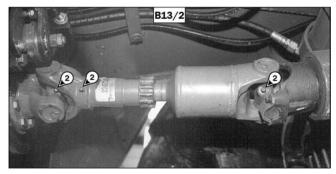
3- Grease fittings for the universal joint between the transmission and rear axle (3) (fig. B13/3).
