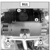
Place a container under the drain plugs (1) (fig. D11) and unscrew the plugs.
