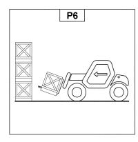
**○** Apply the parking brake and set the forward/reverse lever in neutral.
