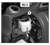
Visually check that there is no leakage at the reservoir and connections.
