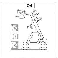
⇒ If this is not possible, back up the telescopic handler (1), maneuvering very gently and carefully to release the load. Retract (2) and lower the boom (3) to bring the load into the transport position (fig. O5).
