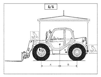
Place the hooks in the fastening points provided (fig. 1/2 and 1/3).
