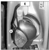
Connect the quick-connectors as needed for the attachment's hydraulic movements.
