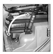
To prevent inadvertent release, the lever is fitted with a safety lock.
