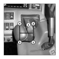
To shift gears, it is necessary to cut off the transmission by pressing the button (1) on the shift lever.
