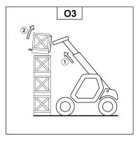
→ Tilt the load sufficiently rearward to ensure its stability.
