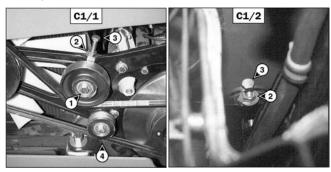
**IMPORTANT:** When changing the fanbelt, tighten screw (3) (fig. C1/1 and C1/2) one-and-a-half turns, after having allowed the engine to idle for 30 minutes.
