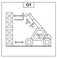
Stop the forks in front of the load by alternately raising and extending the boom (1) or, if necessary, moving the telescopic handler forward (2) (fig. O2). Apply the parking brake and shift the transmission into neutral.
