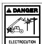
Keep machine, boom and load 10 feet (3 m) or more away from power lines.
