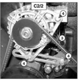
**IMPORTANT:** If the alternator belt is replaced, check the tension again after 20 hours of operation.
