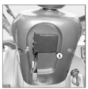
This handle enables the angle and height of the steering wheel to be adjusted.
