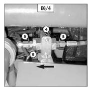
**IMPORTANT:** Be sure to install filter (6) (fig. E6/4) in the same direction as the arrow.
