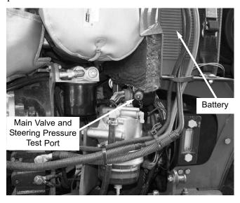
**Battery:** The battery is located under the engine cover toward the front of the engine compartment directly to the rear of the air cleaner.
