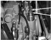
Release Screw Jam Nut
