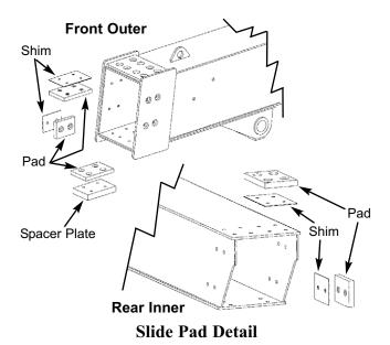
Visually check for loose pad bolts. The bolts are torqued to 30 ft.-lbs. (40 Nm). If the bolts are retorqued at any time, Loctite® 271 (red) thread lock must be re-applied to the bolts.
