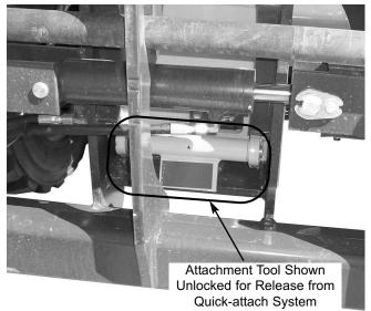
**Quick-attach System Detaching Detail**
