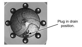
**IMPORTANT:** DO NOT discharge oil onto ground. Catch and dispose of per local waste disposal regulations.
