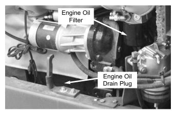
**IMPORTANT:** DO NOT discharge oil onto ground. Catch and dispose of per local waste disposal regulations.
