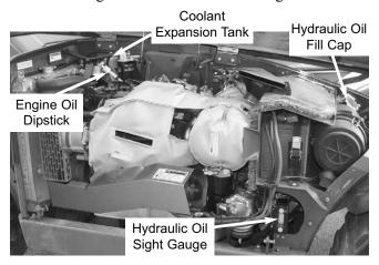
**Engine Oil Level:** The yellow dipstick is located on the top of the engine about centered above the valve cover.
