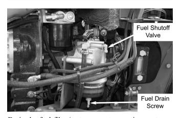
Drain the fuel filter/water seperator anytime water or other contaminants are present.
