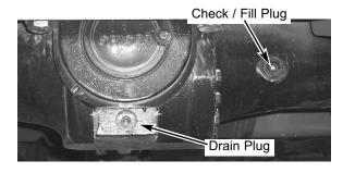
**IMPORTANT:** DO NOT discharge oil onto ground. Catch and dispose of per local waste disposal regulations.
