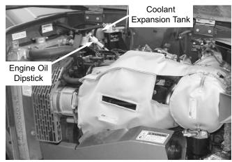
If the coolant is below the Add mark on the tank, remove the cap and add a low-silicate ethylene glycol based coolant mixed with quality water and supplemental coolant additives (SCAs) suitable for heavyduty diesel engines to the coolant expansion tank. See the engine manual for additional information. Replace the cap securely.
