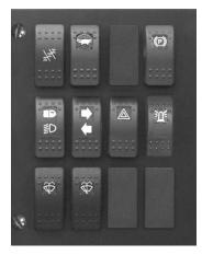
The switch panel contains three rows of switches for the operation of standard and optional equipment on the telescopic handler.
