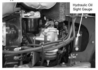
**IMPORTANT:** Be careful when removing the reservoir filler cap so that no dirt or other foreign matter enters the hydraulic system. DO NOT OVERFILL.
