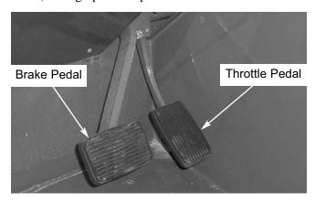
Service Brake Pedal and Transmission Cut-off: Pressing the brake pedal hydraulically activates the internal braking mechanism in the front axle. During initial brake pedal travel and as the brake pedal is pressed farther, power to the transmission is progressively cut off. This allows faster engine speeds at slower operating speeds while maintaining power to the hydraulic system.
