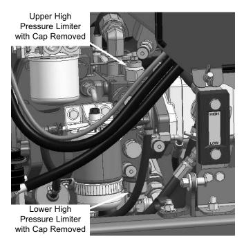
2. Loosen the jam nut on a high pressure limiter.
