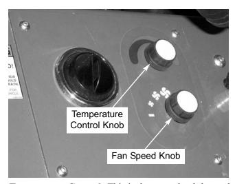
**Temperature Control:** This is the upper knob located to the left of the steering wheel. This knob is used to adjust the temperature output of the heater. Turning the knob clockwise will increase the temperature output of the cab heater.
