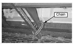
**NOTE:** The PWP must meet ANSI/ASME B56.6-2002, Section 8.24. (See page 13 in the Safety chapter for PWP design requirements.) If the PWP being used does not offer means to secure the PWP to the forks and to secure the forks from pivoting, as shown in Steps 2 and 3, then an alternate method must be used.
