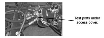
Before conducting any test port pressure checks, check the engine RPM. Engine speed must be 800 RPM at idle and 2500 to 2550 RPM at high idle.
