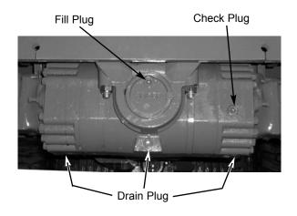
**IMPORTANT:** DO NOT discharge oil onto ground. Catch and dispose of per local waste disposal regulations.
