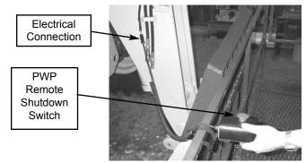
Remote Shutdown Switch With Coiled Wire Connector
