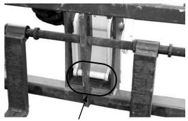
Attachment Tool Shown Locked to Quick-attach System
