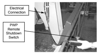
Remote Shutdown Switch with Coiled Wire Connector
