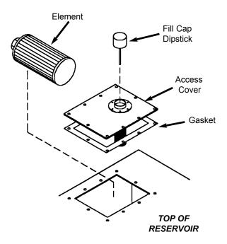
**Hydraulic Reservoir Sump Strainer Removal**
