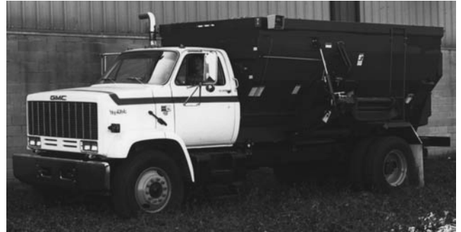
Fig. 1: Typical Truck-mounted Mixer Feeder
