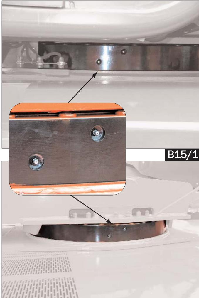
**B15 - Clean and lubricate the turret's fifth wheel coupling**
