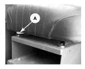
Suspension Seat Option: In addition to the "A" latch handle for forward and rearward adjustment, this seat has a knob "B" under the front of the seat to adjust the suspension.
