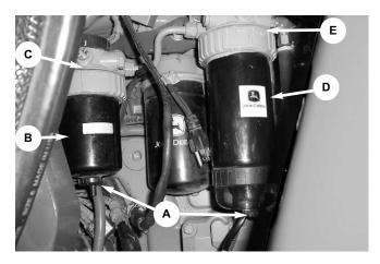
**NOTE**: The engine is equipped with a water-infuel sensor at the primary fuel filter (D). An error code will display in the multi-function display.
