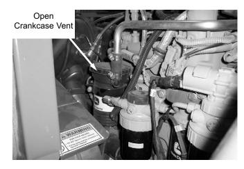
Located near the final fuel filter, the open crankcase filter element should be replaced by:
