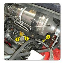
In case of use in a heavily dust laden atmosphere, there are pre-filtration cartridges, see: 3 - MAINTENANCE: FILTERS CARTRIDGES AND BELTS. Also, the checking and cleaning periodicity of the cartridge must be reduced (up to 250 hours in a heavily laden dust atmosphere and with pre-filtration).
